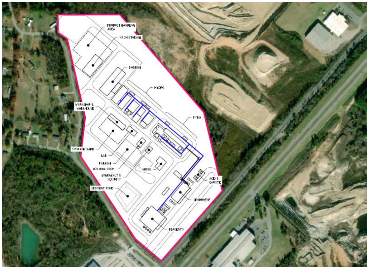
Figure 17 – Indicative Site Plan of Piedmont's Proposed 22,700 tpy Lithium Hydroxide Plant
