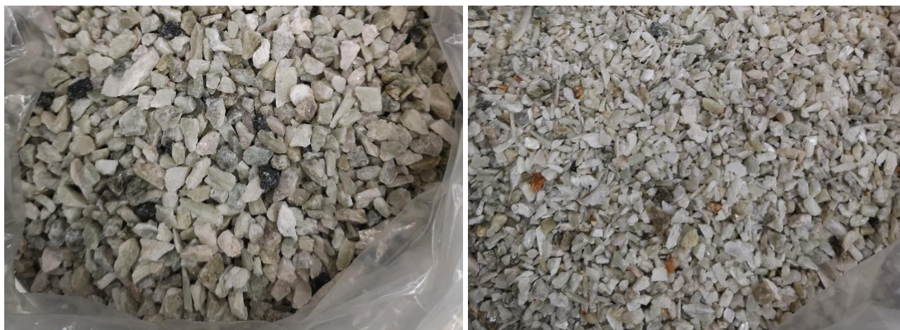
Figure 6 - Coarse and fine final DMS concentrates produced from Piedmont composite samples
