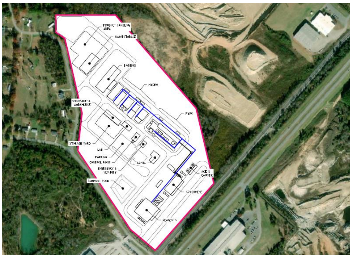
Figure 14 – Indicative Site Plan of Piedmont’s Proposed 22,700 t/y Lithium Hydroxide Plant
